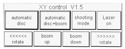
All functions for 360° shots are available. In case of solo mode, the button **"automatic disc+boom"** is out of service.
